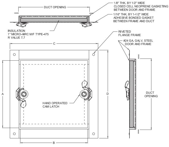
STANDARD FEATURES: REMOVABLE DOOR PANEL, SELF TIGHTENING HAND OPERATED CAM LATCH, GALVANIZED STEEL, MILL FINISH.
