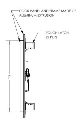
FOR WALL INSTALLATION, HINGE SHOULD BE LOCATED AT BOTTOM
