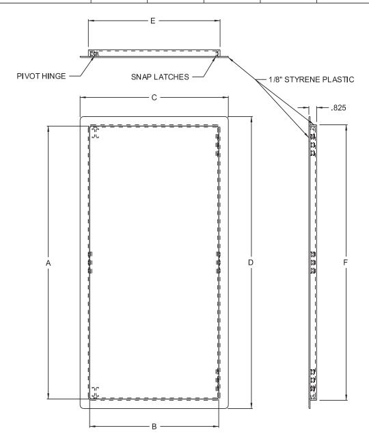
STANDARD FEATURES: HINGED DOOR PANEL WITH SNAP LATCHES, HIGH IMPACT STYRENE PLASTIC WITH U.V. STABILIZERS, WHITE WITH TEXTURED EXPOSED SURFACES
