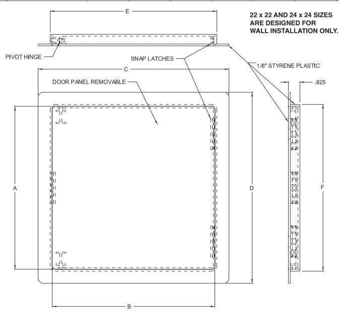
STANDARD FEATURES: HINGED DOOR PANEL WITH REMOVABLE FEATURE, SNAP LATCHES, HIGH IMPACT STYRENE PLASTIC WITH U.V. STABILIZERS,
