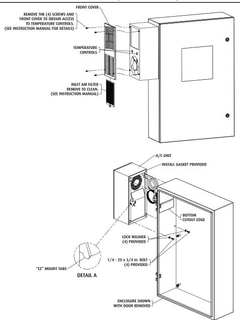
After enclosure has been mounted to the wall, the A/C unit can be mounted to the enclosure.
