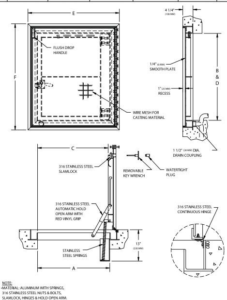
316 STAINLESS STEEL NUTS & BOLTS, SLAMLOCK, HINGES & HOLD OPEN ARM. -LOADING: 300 LBS. PER SQ. FOOT.
