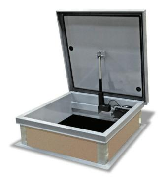
**Opening:** Convenient electric actuation with options of Push Button Switch, Key Switch and/or Remote Control. Can be kept open at any angle for ventilation. Single covers with more than one actuator operate on synchronous mode. Hatches with more than one cover have at least two actuators which need to be operated in sequence. Battery back-up is provided for emergency exits to ensure power supply in case of power outage. Control Box keeps the batteries charged.
