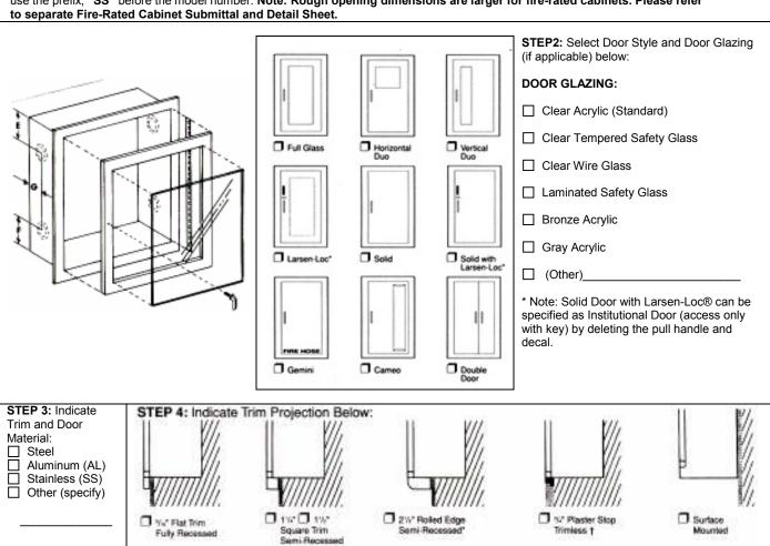
† Trimless cabinets must be installed before the drywall because their plaster stops must be behind the drywall. Trimless cabinets are not recommended for block wall installation.
