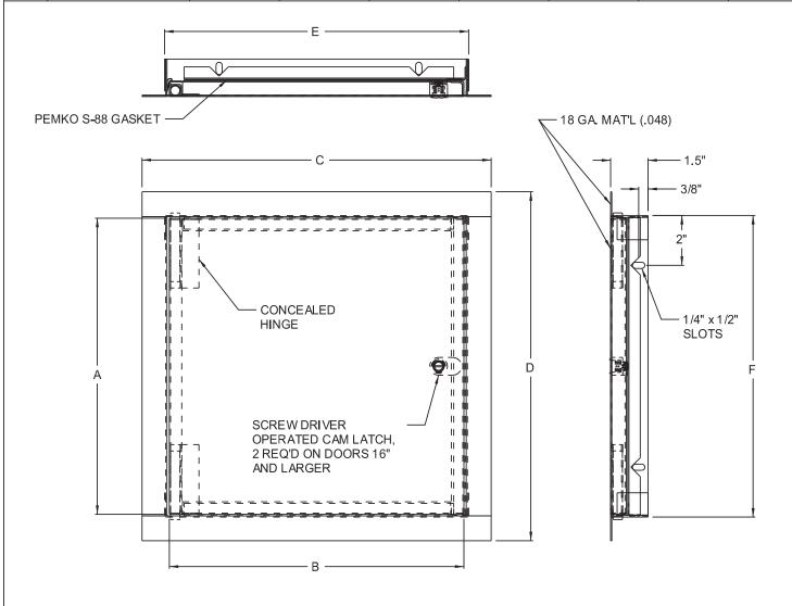
STANDARD FEATURES: SCREW DRIVER OPERATED CAM LATCH,
